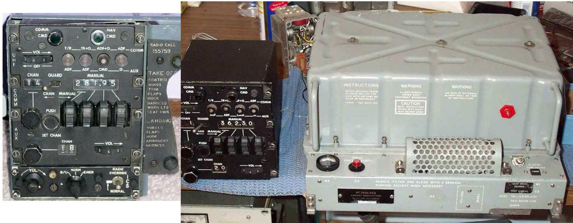
**ARC-109** has AM en DSB, 30W RF, in about the same box as the ARC51.
