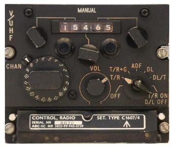
**C1607-4 / PTR175**, made by Plessey. They added 350 VHF channels to the ARC52. Consequently, the 100MHz knob in the control panel can be set to 1, 2 or 3, not only 2 or 3. Further, a veeder type display is used for the manual frequency like in the ARC52.
