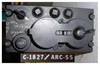
**C-1827**/ **ARC-55** is a simple control without preset channels. It was designed for the ARC55, the non-pressurized version of the ARC27.
