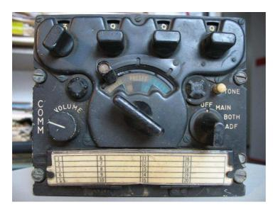
The ARC34C had 50kHz channel spacing. The rightmost rotary switch on the control panel had 20 positions, and the tiny window above that knob showed .00 .05 .10 .15 etc. There was no remote indicator for the ARC34C as far as I know.
