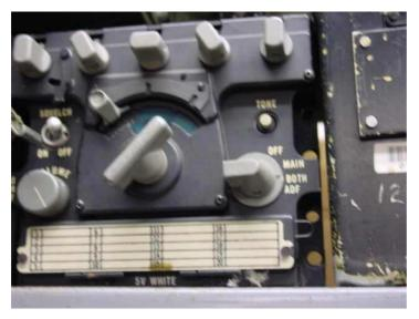
Maybe this control was also used for the ARC34C. It has a fifth knob for the 50kHz channel separation.
