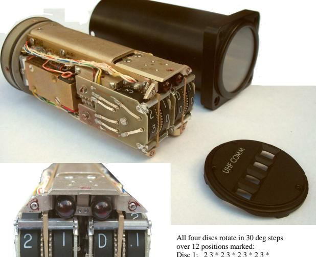
All four discs rotate in 30 deg steps over 12 positions marked: Disc 1: 23 \* 23 \* 23 \* 23 \*Disc 2: G 0 1 2 3 4 5 6 7 8 9 \* Disc 3: D 0 1 2 3 4 5 6 7 8 9 \* Disc 4: \* 0 1 2 3 4 5 6 7 8 9 \* \* no character Illumination by 6 (red) lamps 4.5V/65mA, 1 inside each disc, and two on top to illuminate "UHF COMM"
