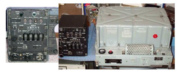
**ARC-109** has AM en DSB, 30W RF, in about the same box as the ARC51. Components shown below C-6364/ARC109 en RT-749/ ARC109
