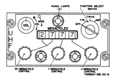
Figure 2-1. Radio Set Control C-4677/ARC-51X, front panel controls.
