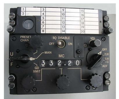
Compared to the ARC34 control, a squelch disable was added, and readout of the manual frequency is far better.
