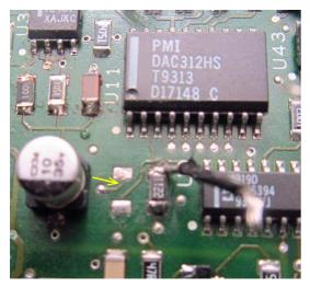
Clearly, the analog sweep was not converted correctly into digital numbers that address the memory. Conversion is done with a 9 bit up/down counter, driving a current output DAC. Its 0...4mA output current is fed thru a 1.25k resistor and compared with the 0...5V analog sweep sawtooth. Deviation of more than 50mV give up or down pulses to the counter.
