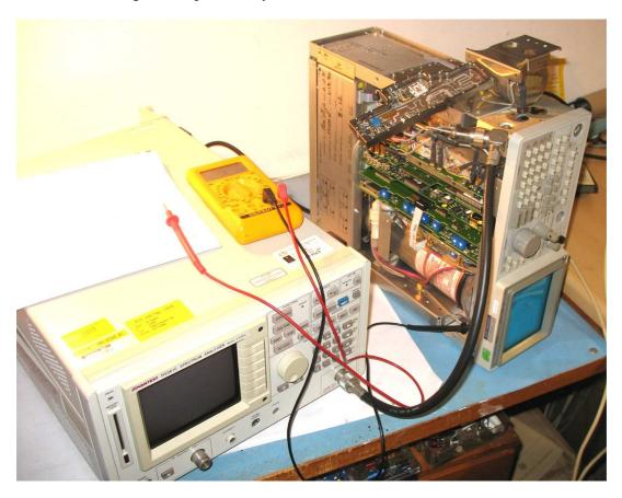
The buffer is a single stage GaasFet, with stabilized output power. Stabilisation is done by rectifying the RF output, an opamp compares this with a blue potmeter reference. The opamp drives the drainvoltage of the Gaas FET via a transistor.
