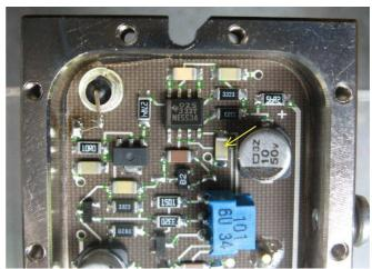
I hope the detector diode is not damaged by the 7V reverse voltage. This type of schottky diodes has a maximum reverse voltage of 4V, but there are no signs even after 2 years, only a higher 0Hz peak.
