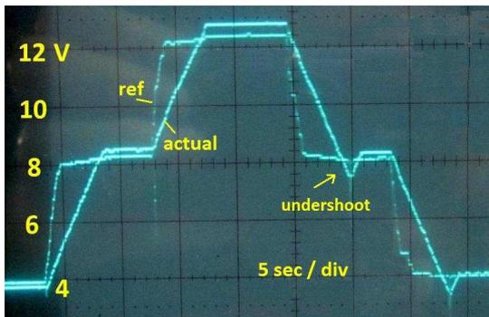
The position of the tuning elements is measured with a potmeter, producing a voltage between 1.7V ( approx. 240 MHz) and 22V ( approx. 193 MHz). The channel selection in the control panel provides a voltage in the same range. When the difference between these two voltages is more than 0.1V, the motor runs either forward or backwards.
