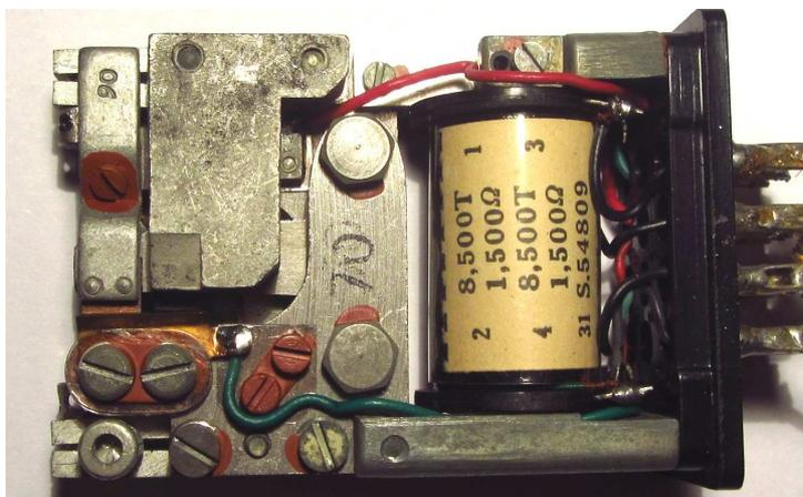
The sensitivity of this relay is remarkable: 0.12mA x 0.4V with both coils in series is 0.05 mW !!
