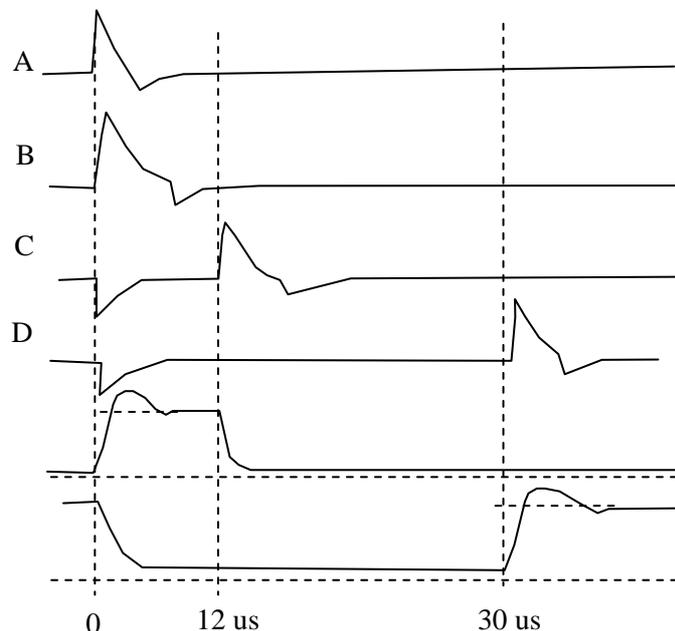
**Pulse D** checks if the received pulse is longer than 30us, to produce a 1 kHz tone during a dot or dash of the beacon identifier (ID). Eureka beacons normally respond with short (5us) pulses. However, every few minutes a beacon ID is transmitted as a two-letter morse code by widening the response pulse to 33us during the dots and dashes.
