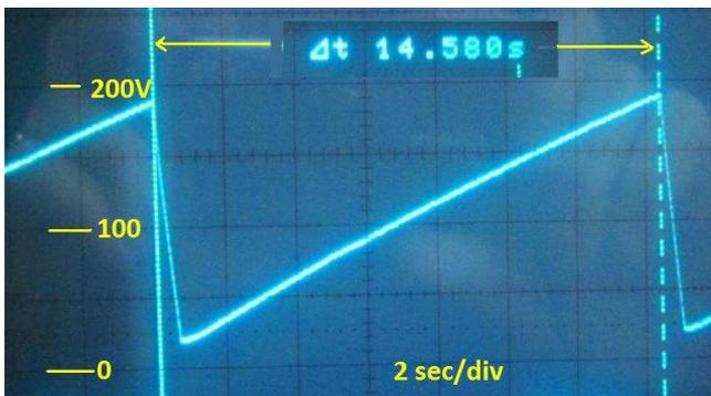
**The 200nm search cycle** takes 14 sec with a 0.5mA range meter connected ( and 150k extra series resistor). Without meter the cycle takes only 12 sec (!)
