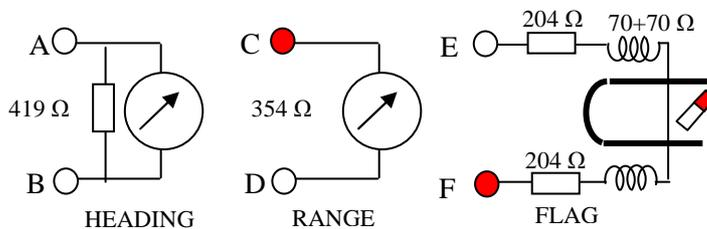
The Heading moving coil is shunted with resistor to get 100uA in either direction.
