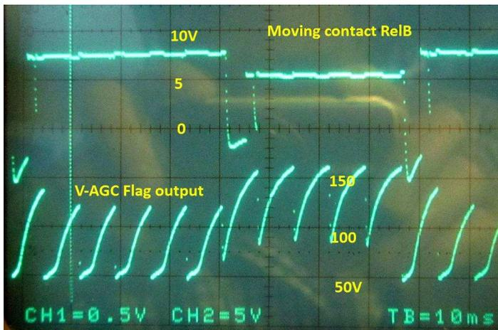
The upper trace in this recording is the voltage  $V_x$  in the diagram shown above. You see alternating the voltages  $V_a$  and  $V_b$  here, and during the change-over time of the lobe-switching relay the voltage  $V_g$  which -amplified by V11a - controls the gain of the IF amplifier.
