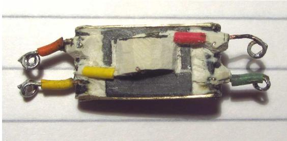
It is nearly impossible to re-wind the original transformer because the ferrite core is brittle, and glued inside the bobbin.
