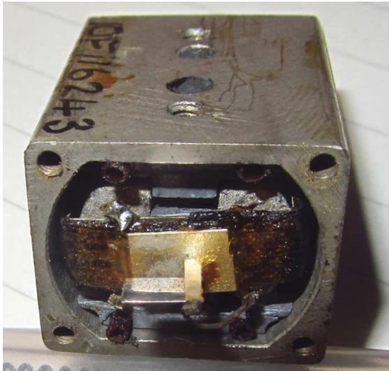
The coil has two separate windings of 350  $\Omega$  each. If the current in both coils in series in either direction is:
