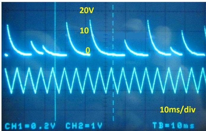
The jitter of the strobe pulse is about 3us, corresponding to 0.3nm. This is not visible on the meter.
