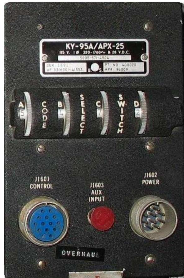
The coder KY95 receives its power supply ( 115Vac and 28Vdc), as well as the decoded mode 1, 2 and 3 pulses ("challenges") from the RT279/APX unit via the 10-pin plug J1602 "power". The coded reply is sent back to the RT279 via this plug as well.
