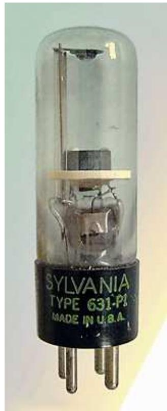
The 631-P1 illustrated was a Sylvania Electric Products device. Basic operating details are: Anode Voltage: 220 - 380 VDC, Trigger Voltage: -70 VDC, Typical Anode Current: 100 mA. The base was UX4 and the grid was a graphite ring. Maximum flash rate: 200 Hz. Produced from about 1950.
