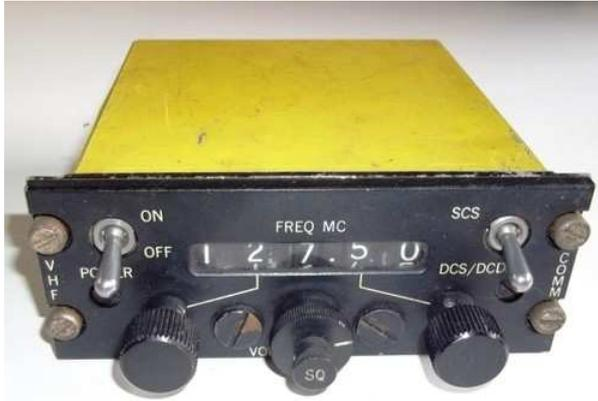
**614U-1** with Single Channel Simplex(SCS) or Dual Ch. Simplex or Duplex (DCS/DCD) switch.
