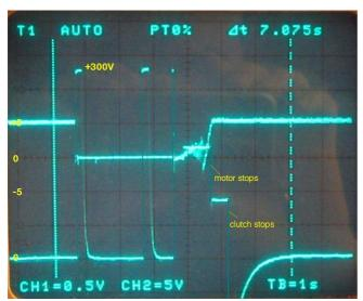
In this picture, the upper trace is the voltage on the top of the gearbox coil, the lower trace is the dF error.
