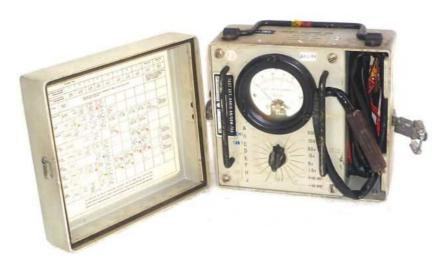
These are measured with the URM-76A voltmeter for a quick go/no-go test on each of the 9 modules in the ARC-34. Each test connector is color coded.
