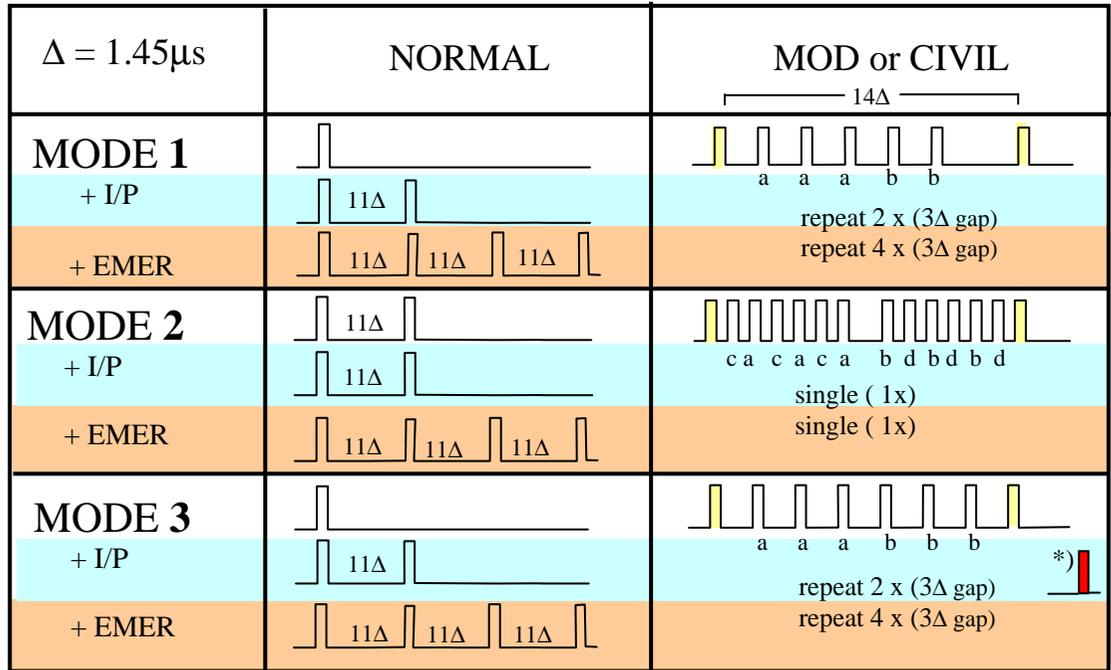
\*) extra pulse 3Δ after mode 3 reply only in CIVIL mode as I/P
